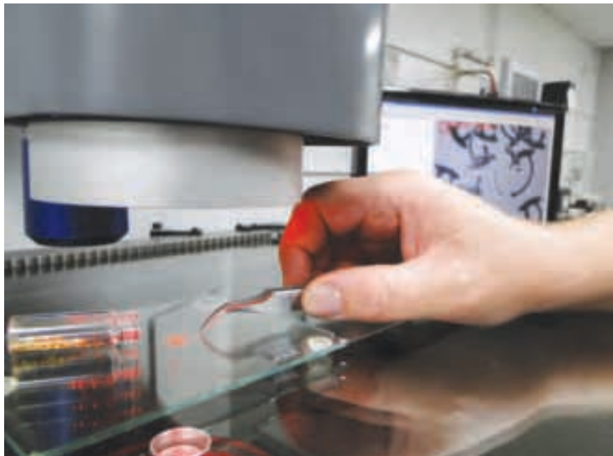
Stamped, gold-plated microparts for an electronic device being inspected on a Brown & Sharpe Optivision system. Closeup of parts (left).
